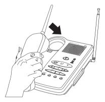
The *charge* LED will blink quickly, indicating that the Digital Code has been reset.
